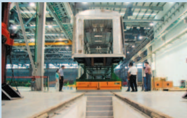
With hydraulic lifting tables components are lifted up to the train for assembly
