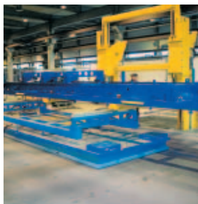
The frame is positioned precisely with the aid of the integral lifting table
