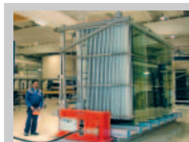
A large amount of glass sheets can be safely moved with the stable radio-controlled Mover
