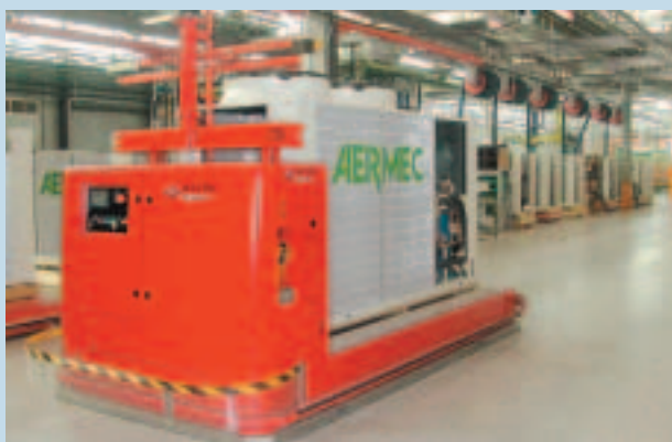
... When it is about to lift the load, it transfers to air bearings to lift the load from the floor
