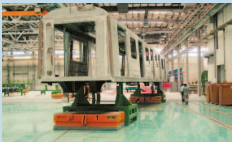
The Mover, floating on air bearings, optically follows the painted line in the floor until it reaches the rails, then it transfers to wheels
