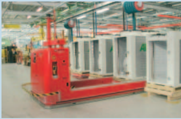
The AGV drives to and from the load on wheels...
