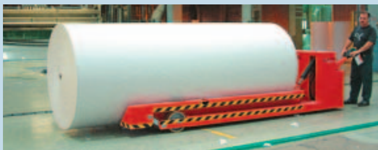
The pallet truck is easily manoeuvred and controlled from the steering arm at the end of the truck.
