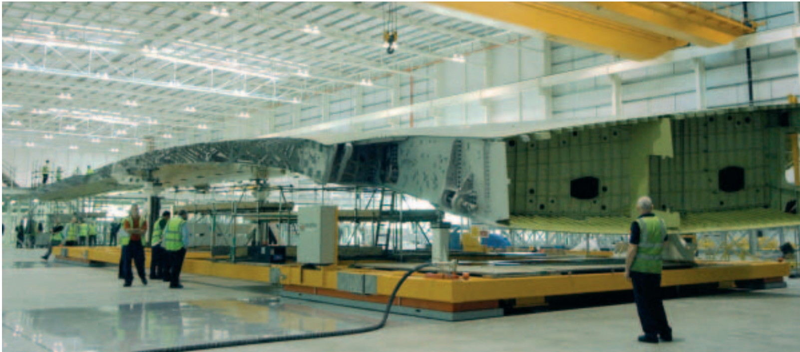
The 40m long wing, seen here from the side, lies on the radio-controlled Solving Platform Mover
